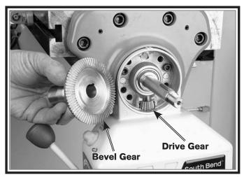
Figure 55. Power feed brass gear and drive gear.
